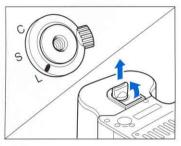
1. Raise the battery case detach lever, turn it in the direction of the arrow towards the "OPEN" side and pull off the battery case.
