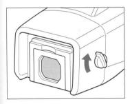
Turn the eyepiece shutter open/close dial in the direction of the arrow.
