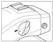
The average light of the entire picture is measured, with emphasis on the center of the picture.
