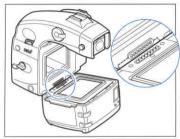
**1.** Remove the camera's rear body cap and the roll-film holder's protection cap.
