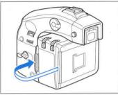
1. Insert the dark slide into the roll-film holder.
