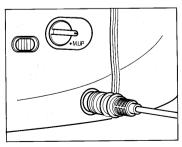
This is the jack for connecting Mamiya electromagnetic cable release (sold separately) when taking photos with the mirror up, with long exposures or with slow shutter speeds.
