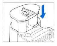
3. Attach the battery case to the camera, then turn the battery case detach lever towards the "
