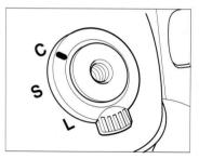
Set the shutter release mode selector lever to "C". Photographs are taken continuously at a rate of about 1.2 frames per second.
