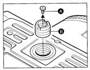
When using a tripod with 3/8 inch screws (larger than the normal tripod screws), remove the small screw (a) from the tripod screw hole on the bottom of the body using a Phillips screwdriver, then use a coin to remove the tripod screw adapter (3).
