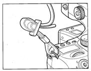
Put the next strap through the camera's strap mount as shown on the diagram and tighten it. For safety, check that the strap is securely fastened to the strap mount.
