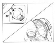
1. Turn the focus mode selector lever, select "M", then turn the lens distance ring to focus.
