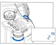
1. Press the mode setting button (A) twice to set the multiple exposure mode.
