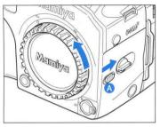
1. Remove the camera's body caps using Lens Release Button (See opposite page) and the lens's front/rear caps.
