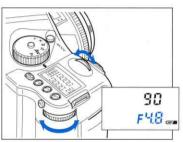
2. Turn the front or rear dial to set the desired aperture.
