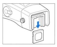
**1.** Remove the diopter corrected lens (DE401) from the camera.
