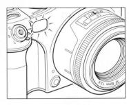
When the subject is dark or the contrast is low and the camera is having trouble focusing automatically, a red lamp may light on the front of the camera when the shutter release button is half-pressed. This is a supplemental light that assists the camera's auto focus function.
