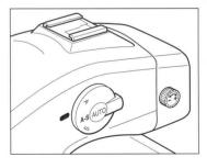
There are three exposure metering modes: "A" in which the average light of the entire picture is measured with emphasis on the center of the picture, "S" in which the light in a spot at the center of the picture is measured, and "A-S" which combines these two to automatically switch the mode according to the extent of difference between the brightness of the light metered in the two modes and sets the distribution ratio of the exposure metering modes within an intermediate range. (See page 43.)
