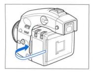
To remove the film roll before the end of film, insert the dark slide in the roll-film holder and press the shutter button and force film advance button simultaneously. This causes the film to be taken up till the end and the LCD panel shows "End".
