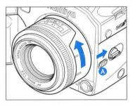
While holding down the lens release button  $extbf{A}$ , rotate the lens in the direction of the arrow until it stops, and release the lens from the camera.
