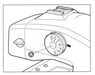
Turn the exposure compensation dial while pressing the exposure compensation dial lock release button  $\triangle$  located next to the viewfinder. The exposure can be adjusted within a range of  $\pm 3$  EV in 1/3 steps.
