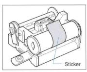
★Move the empty spool from the top to the lower (take-up) compartment, ready for loading the next film roll.
