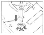
**4.** Connect the power cord from the external battery case to the external power socket.
