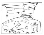
1. Mount the SCA3951 adapter onto the Metz flash, insert fully into the camera's hot shoe, the tighten with the fixing knob .
