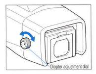
★Point the camera at a bright, plain object such as a white wall when making this adjustment.
