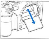
3. Remove the Focusing Screen from the Focusing Screen Frame by grasping the tab on the edge of the screen with tweezers as illustrated.
