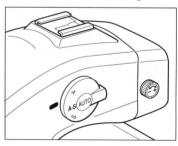
With the average/spot automatic switching exposure metering mode, average or spot exposure metering is selected automatically according to the conditions of the subject and the appropriate exposure is set accordingly.
