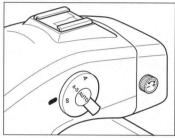
The light in the circle at the center of the picture is measured to determine the exposure. This mode is suited for subjects in which contrasts are strong and when you want to measure the light of certain section of the picture. When the spot you want to measure is not at the center of the picture, use the AE lock function.(see page 55 AE Lock Mode)
