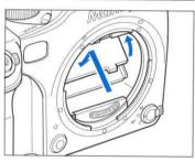
**4.** In case of attaching, insert your desired Focusing Screen to the Focusing Screen Frame properly and then raise the frame until it clicks.
